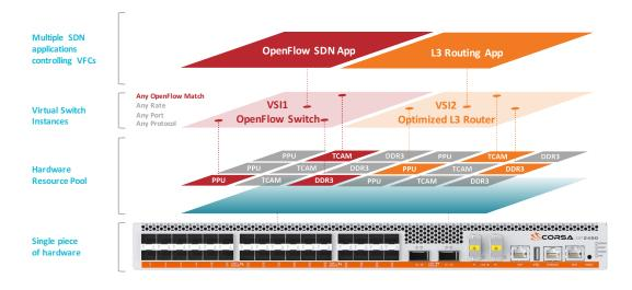
Figure 2: Corsa DP2400 high level architecture presenting two VSIs
