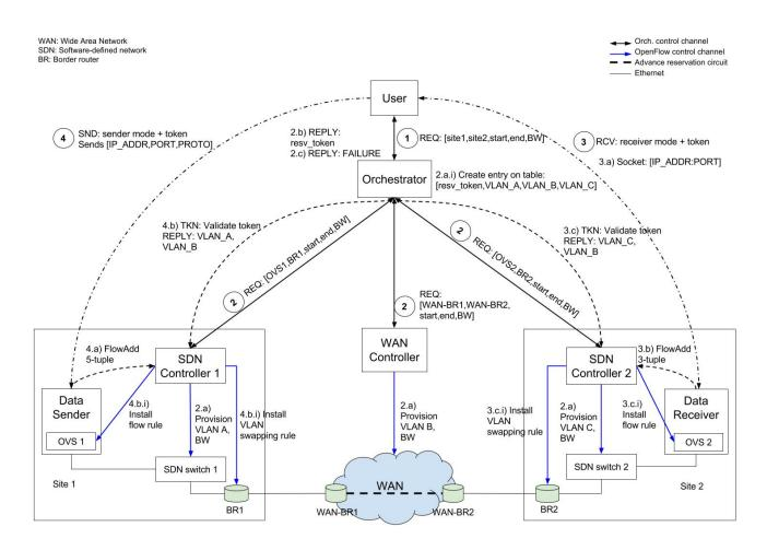
Figure 2: Block diagram of advance reservation access control using SDN and tokens. Only positive outcomes are shown
