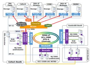
Figure 1: Global Software-Defined Dynamic Circuits for Data Intensive Science – Local and external connectivity.
