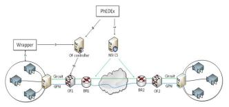
Figure 4: Detailed architecture view in which the ANSE framework is used to request an NSI circuit, with the last mile setup being handled by an OpenFlow solution
