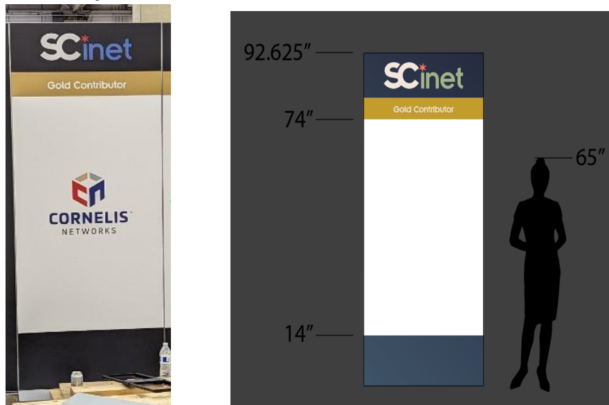
Figure 2: Typical Panels for Contributors and Overall Dimensions
